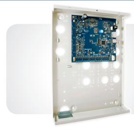
For those sites that require safety checks prior to opening, the panel can automate an area search process which reports a message to your monitoring service if the search has failed to complete on time. Add to this, an extended range of input testing and reporting features where individual inputs can be automatically tested with normal operation within a specified number of days and you have one of the most feature-rich intrusion detection systems available.
